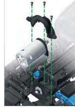
motor pinion (9-T - 22-T) and spur gear size (39-T or 45-T). Remove the two screws from the motor/motor plate and reinstall in the corresponding positions; reinstall the motor/motor plate assembly in the chassis.
