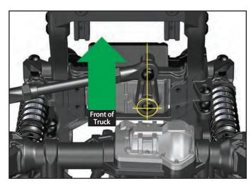
If you are using aftermarket servos, it is important to use servo horns designed for TRX-4. The servo horns must measure 22mm from the steering linkage mounting hole to the servo mounting hole.
