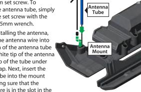
antenna mount; then, install the set screw next to the antenna tube. Use the supplied 1.5mm wrench to tighten the screw just until the antenna tube is securely in place. Do not over tighten. Do not bend or kink the antenna wire! See the side bar for more information. Do not shorten the antenna tube.
