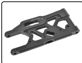
C-00180-010 Suspension Arm - Lower - Rear - Composite - 1 pc
