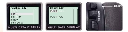
D/R is used to change the action range of steering servo when turning the steering wheel. Increasing D/R will make the steering wheel action more sensitive.
